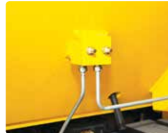
Grease Fittings Grease fittings are installed for fast access to steering axle center pin when doing your service checks.
