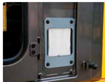
Cabin air fresh filter The internal pressure is maintained to be slightly higher than that of outside to exclude dust and to reduce noise levels.
