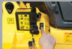
Cabin tilting automatic system Cabin tilting automatic system makes servicing of all power train components quick and easy. An electrically assisted hydraulic actuated cylinder tilts operator cabin to left side about 54 degrees for easy access to inside of truck components.
