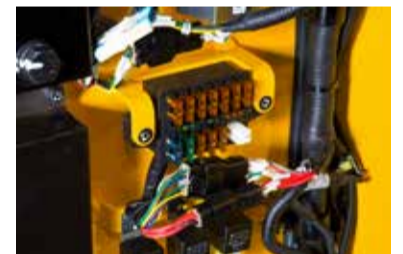
Centralized fuse box
